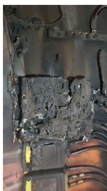
Fig. 11. On 02/05/2023, the main switch installed in the 444kWp photovoltaic plant caused a short circuit followed by a fire in the plant's substation. One of the fuse links did not break, leaving the three-phase circuit energized after the incident.
