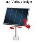
(b) Two tracking Figure 12: Solar collector types
